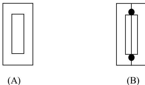
Fig. 2 (A) Rectangular paper template and (B) fibre attached on the frame.
